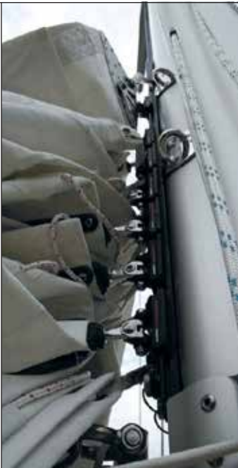
Cut car stack height in half by flaking the sail alternately to port and starboard of the boom.
