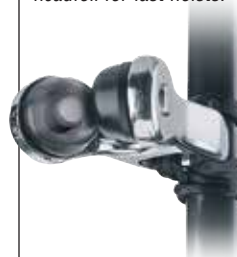
Prefeeder: Hardcoat-anodized, PTFE-coated aluminum rollers spin freely on low-friction bushings.
